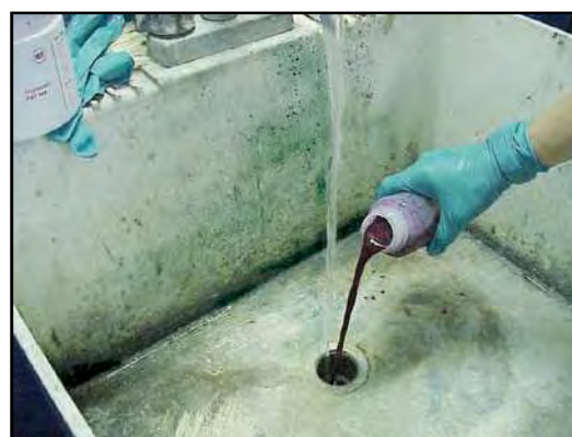
Figure 63: Dye Testing Plumbing (NEIWPCC, 2003)
