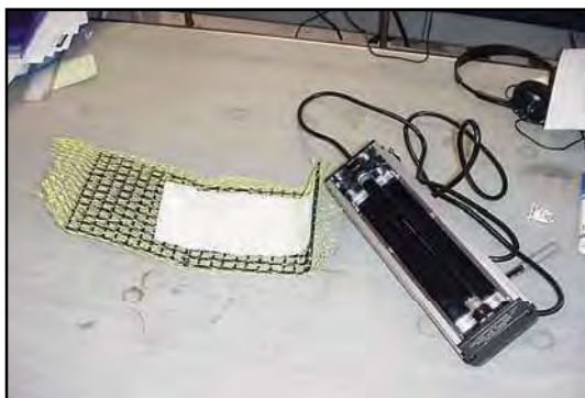
Figure 48: OBM Equipment includes a black light and an OBM Trap that can be placed at an outfall
