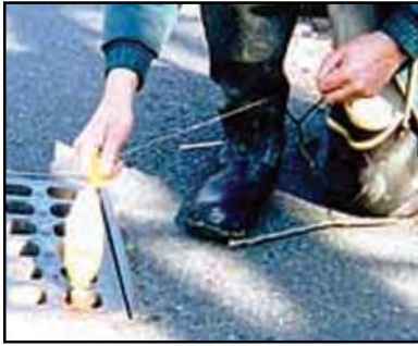
Figure 60: Optical Brightener Placement in the Storm Drain (Source: Sargent and Castonguay, 1998)
